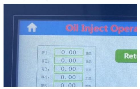
After temp reaches to SV and oil are melt and flow well, then click Return, Finish
