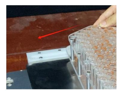
9. Then pull out the metal board as below, until all pre roll go down the sealing tray:
