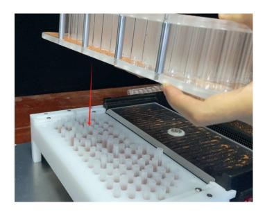
10. Then put NO.6 part on the No.1 sealing tray. And put NO.4 sealing board on the No.6, then press pre roll firmly to sealing pre roll well.
