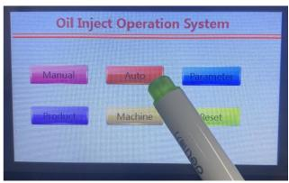
2. How to clean machine (Clean with alcohol when 1st use or after filling)? Pour alcohol into oil tank, Set filling volume at 7ml, click "one" change to be "more." Click <mark>"start";</mark>
