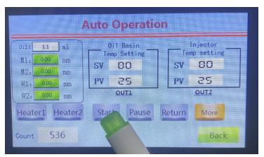
3. After clean air, pour oil into oil tank. Set temp needed, then Click "heater1" "heater2" to heating.
