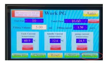
3.2 Set starting temp, and temp setting, starting temp should be lower than temp setting;
