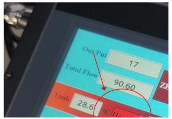
**4, After temp reaches at Starting temp, Clean air** Click Reset, click Clean, it will change it "Cleaning" It will take 10seconds to clean air in the tube and injector
